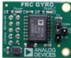
Analog Devices, Gyro Board (am-3555)
